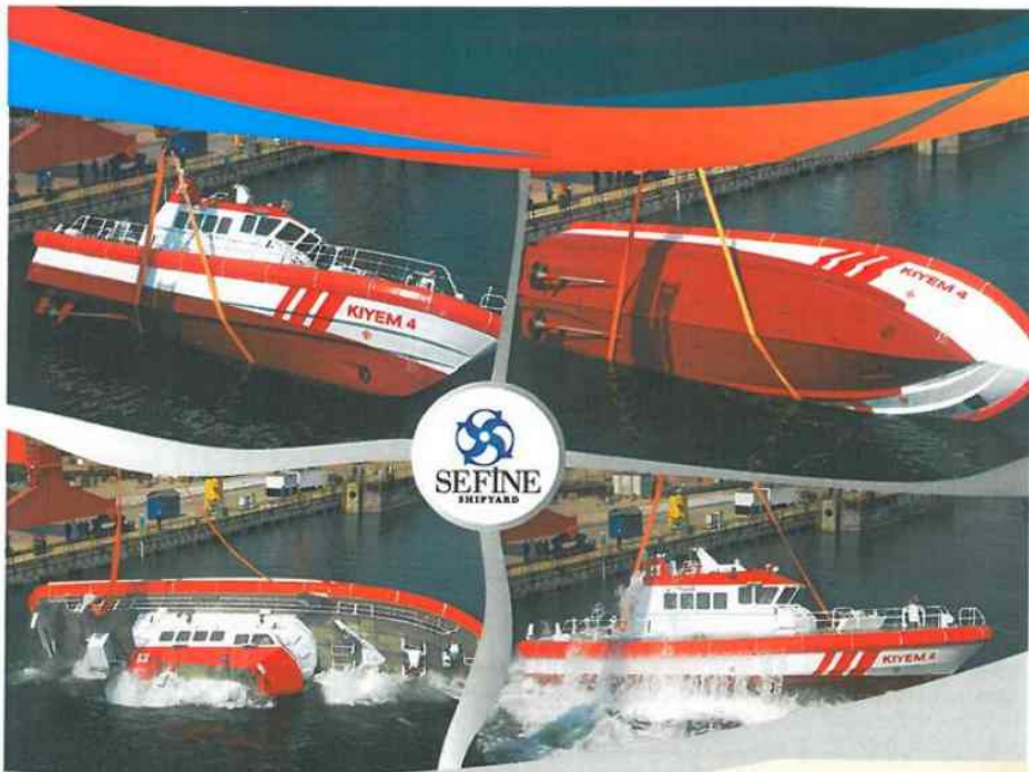
SELF RIGHTING TEST OF SAR BOAT
